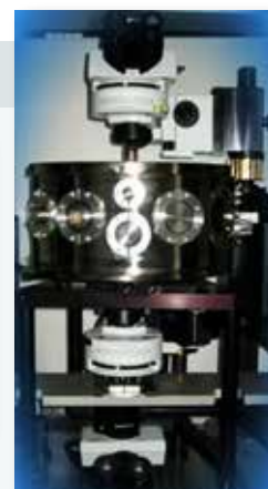
Low temperature SPM system integrated with Raman microscope
