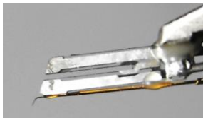
NSOM Probe mounted on tuning fork
