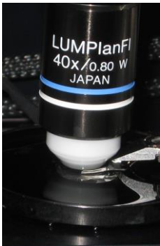
Online integration with Water Immersion Objectives from above for Liquid Cell operation.
