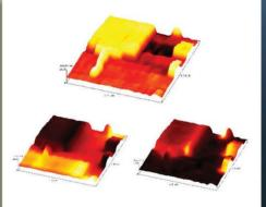
3D AFM topography (top) of a state of the art transistor with on-line pixel by pixel correlation of the Raman spectral distribution of silicon (bottom left) and strained silicon (bottom right). The images represent true chemical distribution since the on-line AFM acts as the finest autofocus mechanism known to date while providing detailed structural correlation.
