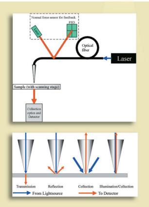
NSOM (SNOM) is the only way to get sub-wavelength optical information from a sample, and as it is usually combined with AFM, the optical information can easily be correlated to topographical information.
