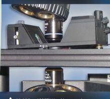
MultiView 1000™ Head integrated with a standard microscope
