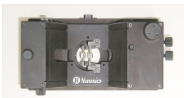
Top View of The Nanonics NSOM/AFM 100 Confocal Microscope™ with Liquid Cell in Place
