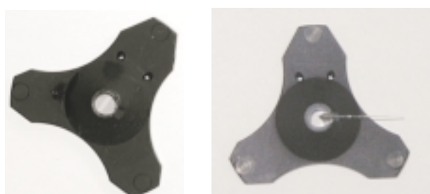
Tip mount with free optical axis. left: without tip; right: with tip mounted
