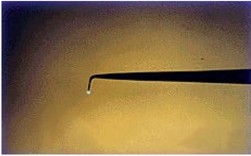
Fig. 2 A Nanonics near-field optical/AFM/electric probe
