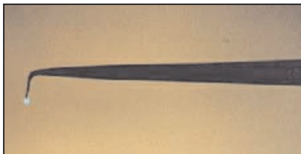
Figure 2 Nanonics cantilevered optical fiber tip
