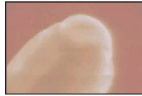
Figure 5 Scanning electron micrograph of a Nanonics probe tip for surface enhanced near-field Raman studies
