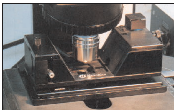
Figure 1 Nanonics NSOM/AFM mounted on a Renishaw RM Series Raman microscope
